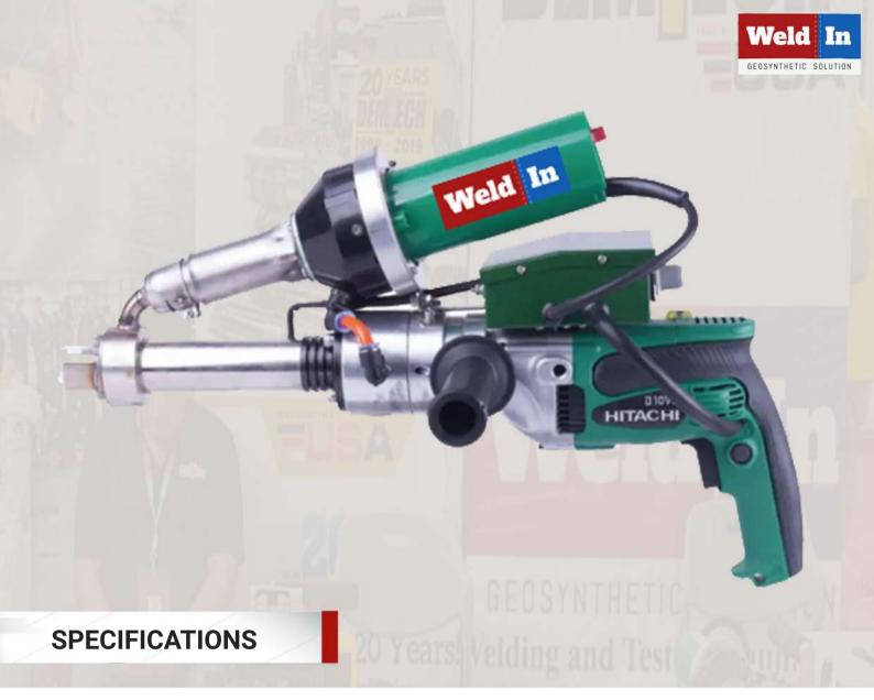
**WIN 600A** Model Rated Voltage 230V Frequency 50/60HZ **Extruding Motor Power** 800W Hot Air Power 1600W Welding Rod Heating Power 800W Air Temperature 20-620 **Extruding Temperature** 50-380 **Extruding Volume** 2.0-2.5kg/h Welding Rod Diameter 3.0-5.0mm **Driving Motor** Hitachi Body weight 6.9kg Certification CE Warranty 1 year
