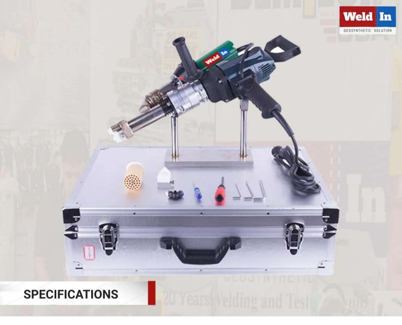
Model Rated Voltage Frequency Extruding Motor Power Hot Air Power Air Temperature Extruding Volume Welding Rod Diameter Driving Motor Body weight Warranty WIN 600F 230V 50/60HZ 1200W 3400W 20-620 Adjustable 2.0-3.0kg/h Φ3.0-4.0mm FEIJI 7.5kg 1 year
