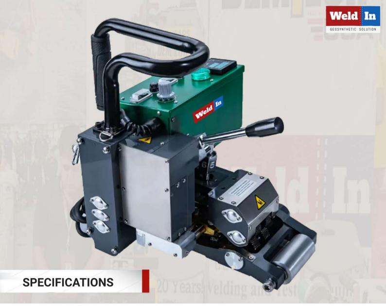
Model Rated Voltage Rated Power Frequency Heating Temperature Welding Speed Material Thickness Welded Seam Width Weld Strength Overlap Width Digital Display Welding pressure Body weight Warranty WIN 900 230V/120V 1800W/1650W 50/60HZ 50~450 1.0-5m/min 1.0mm-3.0mm(single layer) 15mm\*2,Interior Cavity 15mm  $\geq$ 85% material 12cm temperature display 100-1000N 13kg 1 year
