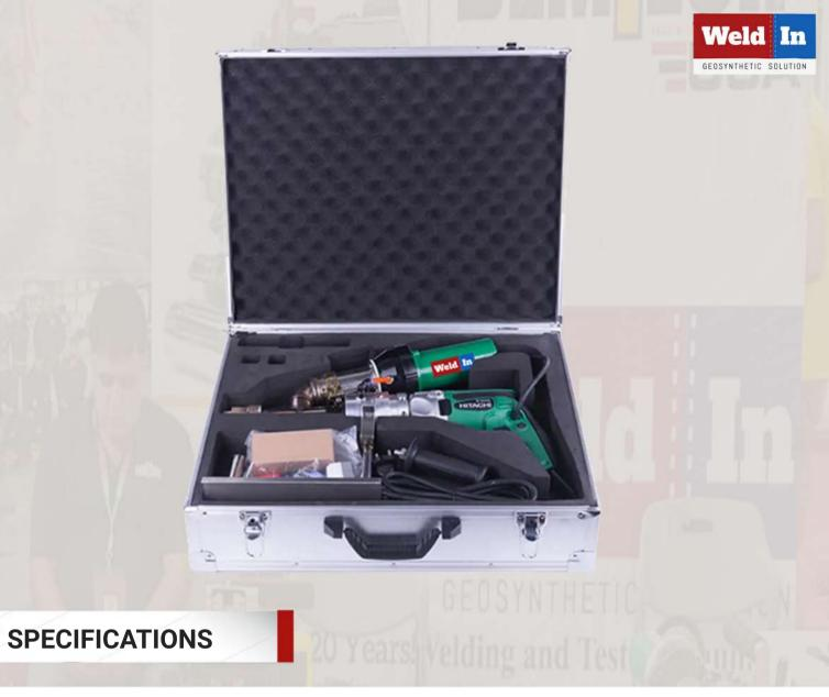
Model Rated Voltage Frequency Extruding Motor Power Hot Air Power Air Temperature Extruding Volume Welding Rod Diameter Driving Motor Body weight Warranty WIN 600E 230V 50/60HZ 800W 3400W 20-620 Adjustable 2.0-2.5kg/h Φ3.0-4.0mm Hitachi 6.0kg 1 year
